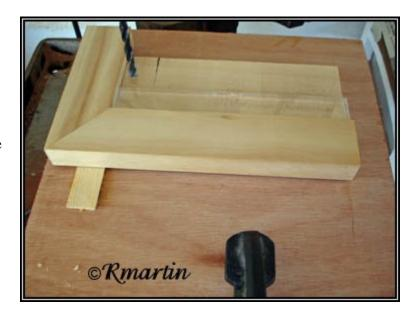
Make sure the inside of the top is face up and the wood grain is aligned with the bottom. Drill the left side hole for each box lid. Rinse and repeat for the right side.
