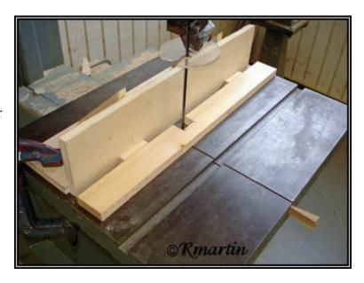
With the rip fence clamped in place, a scrap piece of wood is tested. and at every step in the process. Adjustments are made if necessary and another piece is tested. Once everything is just right, it only takes a few minutes to cut each block of wood.
