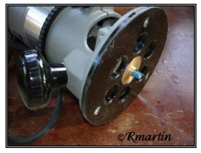
Start by taking no more than a 1/4 inch. Everyone mows the grass a different way. I go around the edges and then pull the router towards me one row at a time. Make several passes until the desired depth is achieved.
