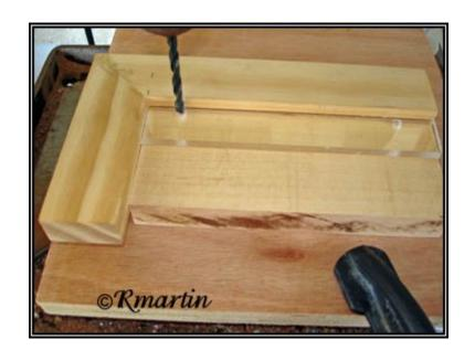
Once the depth stop on the drill press is set, the left side hole of 1 or 100 boxes can be drilled quickly and exactly. Repeat the alignment set-up for the right side hole.
