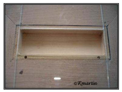
A 1/4 inch round over bit is installed on a dedicated router table. All edges, top and bottom, inside and out, are routered.
