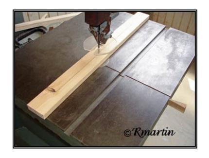
A rip fence jig is made by gluing and screwing together 2 pieces of plywood at a 90 degree angle. Shims are used to set the fence 7/8" from the blade. (Note: I recommend a 1" minimum for the bottom, but I was limited with the wood at hand.)
