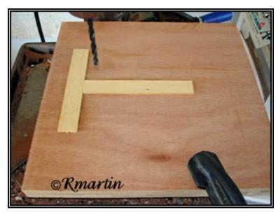
The second jig is made from 3/4" shop stock 1" wide by 12" long. A groove is center cut along one edge. This is done by making a couple passes on the table saw until the mortise is just wide enough to hold a piece of 1/4" plexi glass. Cut on a 45 degree angle and glue in an L shape. Glue in the plexi glass. Lastly, drill two holes in the plexi glass 1" and 5 1/2" from the inside corner.
