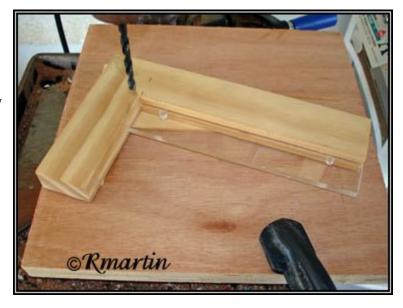
Align the T-base, speed square and drill bit with the bottom of the box. Once everything is nice and snug, clamp the T-base to the drill press.
