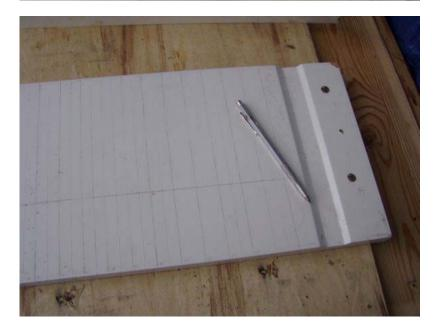
Note that the board is screw on to a waste plywood board, now to have a good edge when cutting I add some scrap wood length on the side and the edges will have a neat cut
