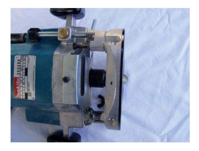
I do plunge cutting and free hand, didn't have the time to do a jig, a safe way to is to use a router table if you got one, depth of the cut is 8.7 m/m or .343" you can do
