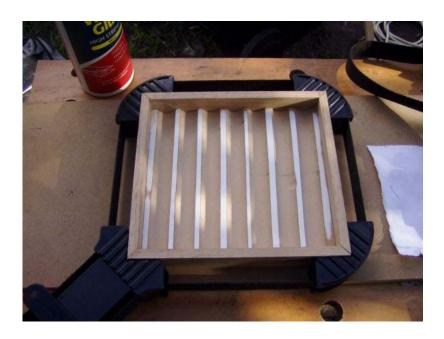
Next I remove the tray from the frame and glue the felt with PVA, I brush the glue then apply the felt and give the shape with a wooden dowel
