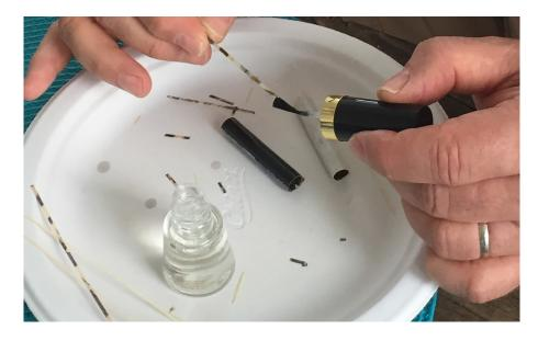
The last strip can overlap to fill the gap without being noticeable. I clean the tube with a paper towel and a little denatured alcohol. Here are the abalone tubes ready for casting.
